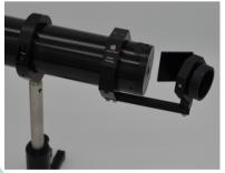
ROM on a HeNe laser with a 1" neutral density filter and light block to capture stray light.
